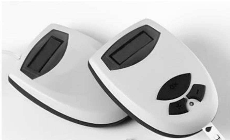
Fig. 2 Commercial glucometer based on an amperometric transducer.
