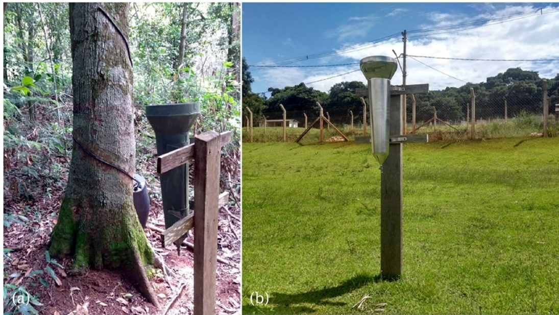
Figure 2. Rain gauge and stemflow apparatus for, respectively, throughfall and stemflow measurements (a) and external rain gauge for gross rainfall measurements (b).
