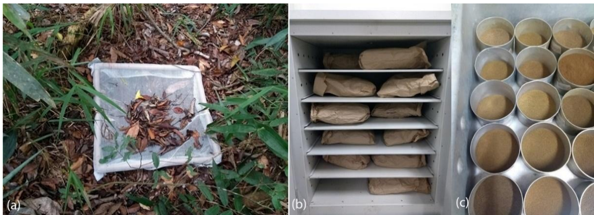
Figure 03. Litterfall deposited during the period between the collections (a), forced-draft oven (b), samples after crushed and sieved (c)
