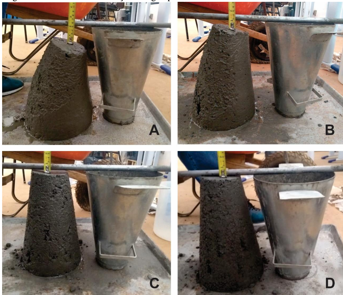
A) Slump test do concreto controle; B) Slump test do concreto 1% BCC; C) Slump test do concreto 3% BCC; D) Slump test do concreto 5% BCC.
