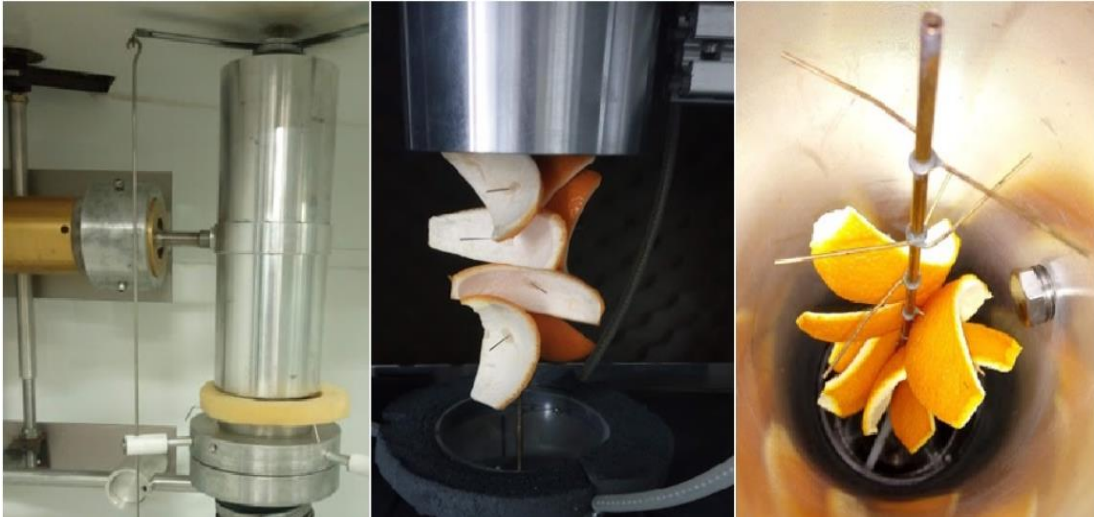
Figure 2 - Cylindrical drying chamber used for the application of ultrasound without direct contact between the emitter and the food. Source: Author (2020).
