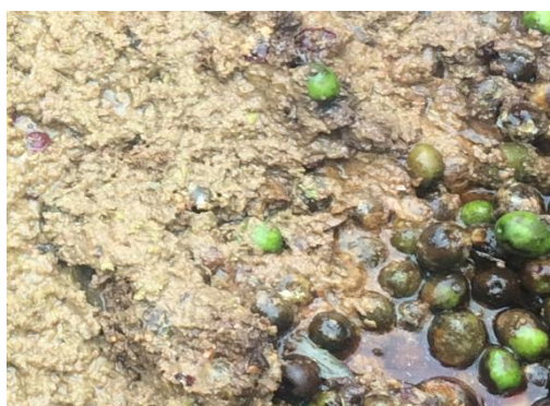
FIGURE 1. Illustrative image of solid residue, alperujo, obtained from the extraction of olive oil by centrifugation system of two phases of Maria da Fé, MG.
