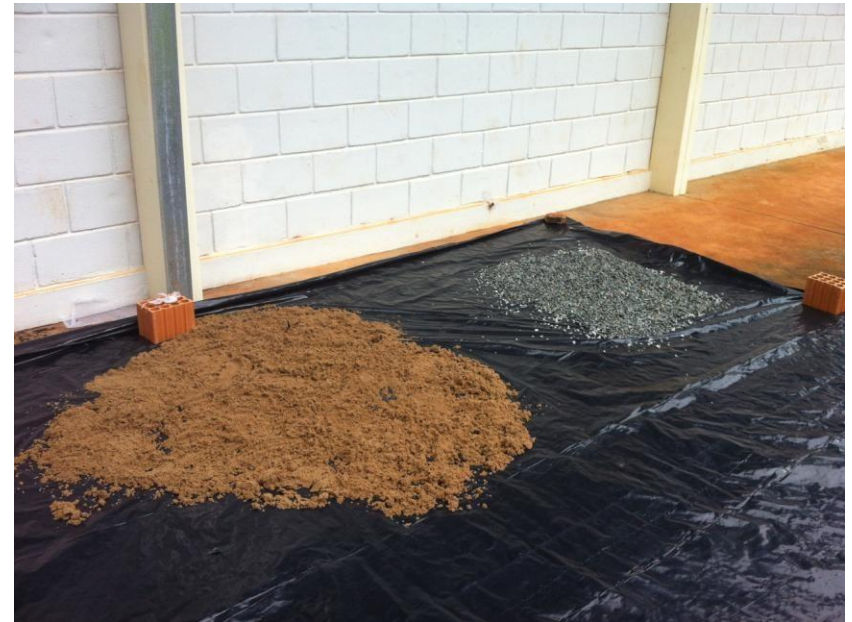
Sand and crushed stone /pebbles drying in the sun after they were washed with a solution of bleach
