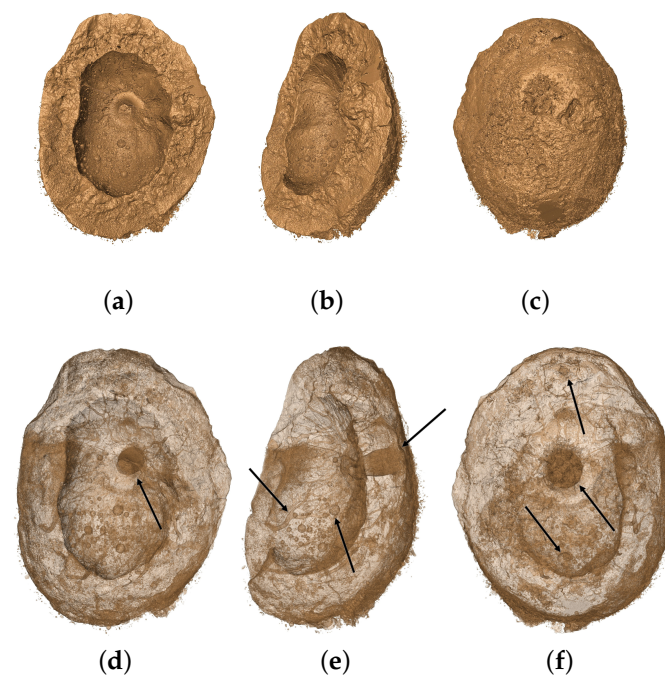
Figure 11. Crushed endocarp's microCT scan images: opaque-colored/translucent-colored volumes' (a,d) inner views, (b,e) lateral views and (c,f) outer views.
