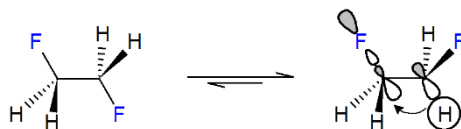
Figure 1. Gauche effect in 1,2-difluoroethane due to \sigma_{\text{CH}} \rightarrow \sigma^*_{\text{CF}} hyperconjugation.
