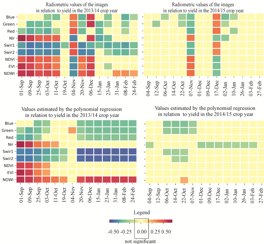
Fig 8. Pearson correlation between Landsat 7 ETM+ and 8 OLI bands and spectral indices with yield using the current and estimated polynomial images for the crop of years 2013/14 and 2014/15.
