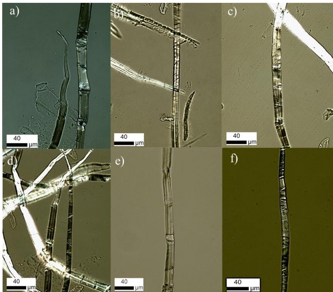
Figure 7. Typical light-polarized microscopic images of Eucalyptus sp. bleached fibers, showing the dislocations in samples with enzymatic pre-treatments: a) control; b) control fibers with heating at 50°C; c) enzyme A; d) enzyme B; e) enzyme C; and f) enzyme D.
