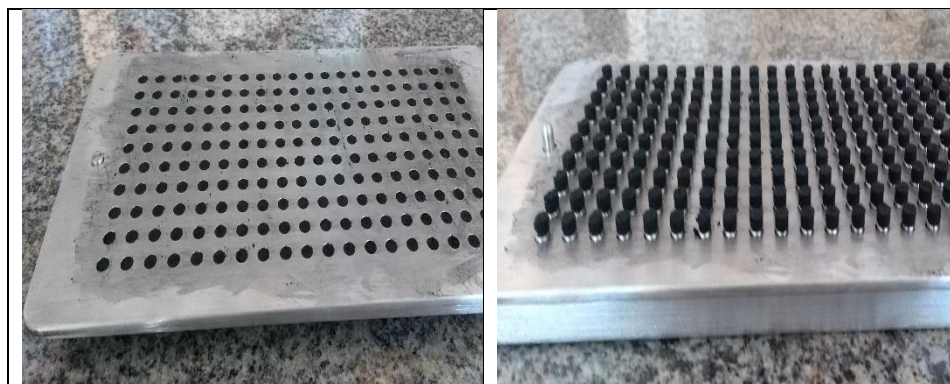
Figure S1. Stainless steel pastillator used for the production of the biochar-based fertilizer granules.
