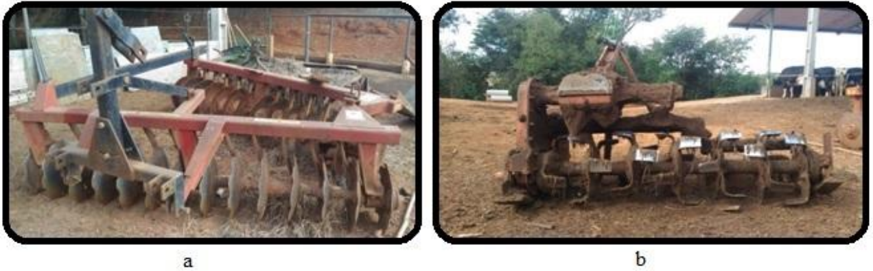
FIGURE 2 - Agricultural implements used to turn the bed. (a) disc harrow; (b) rotary hoe.
